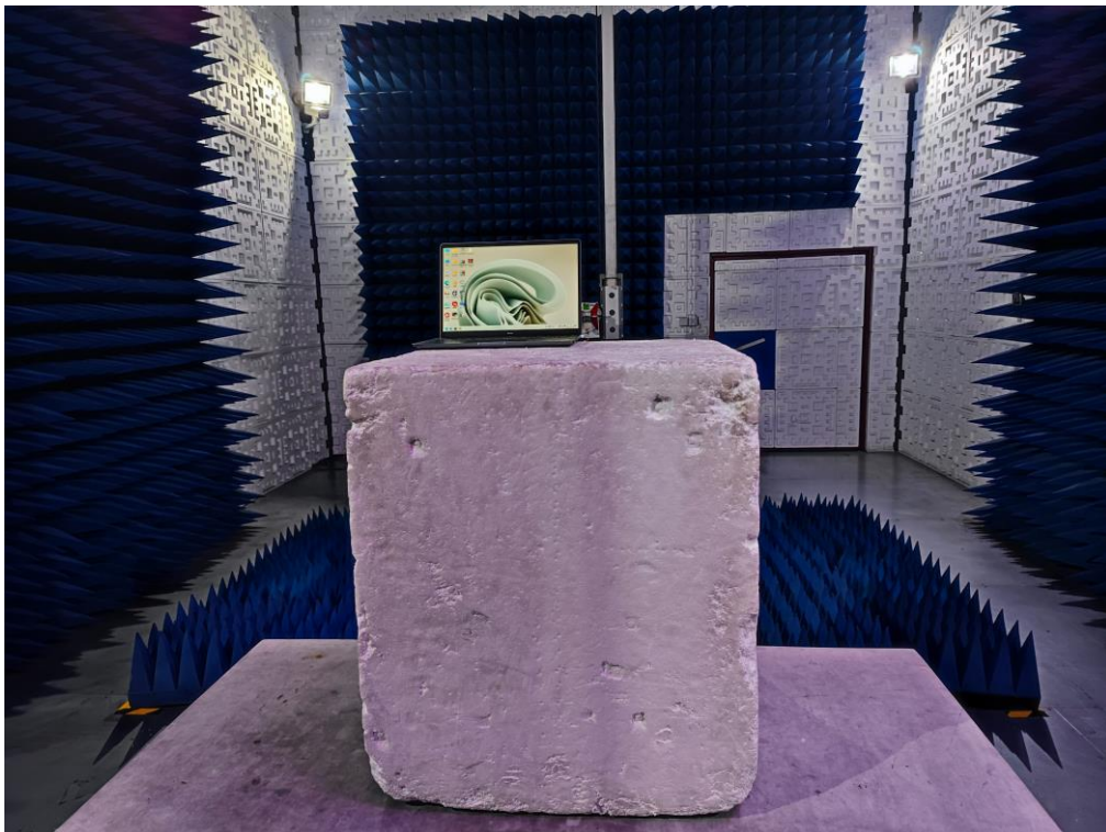
RADIATED EMISSION TEST SETUP ABOVE 1GHz
