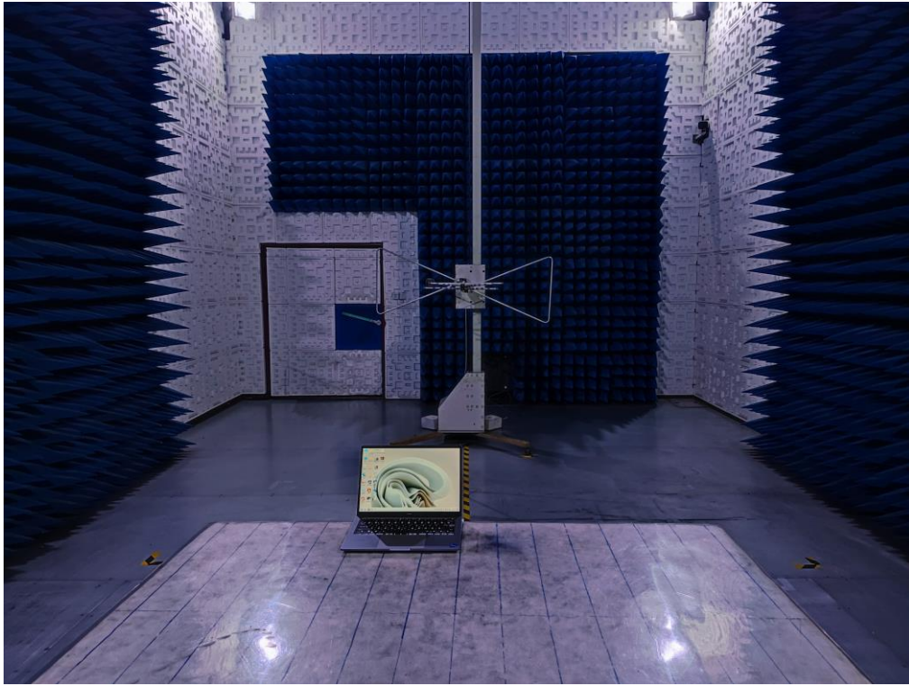
RADIATED EMISSION TEST SETUP ABOVE 1GHz
