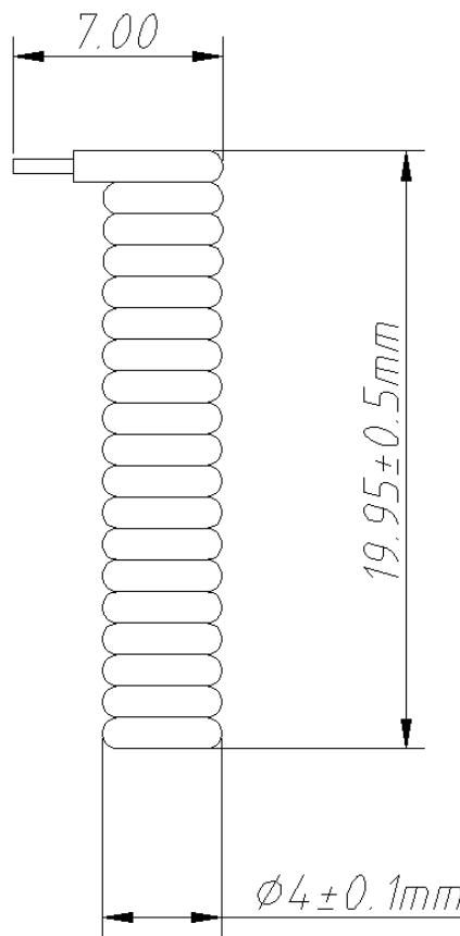
Antenna: Integral antenna with maximum gain of 2.0dBi
