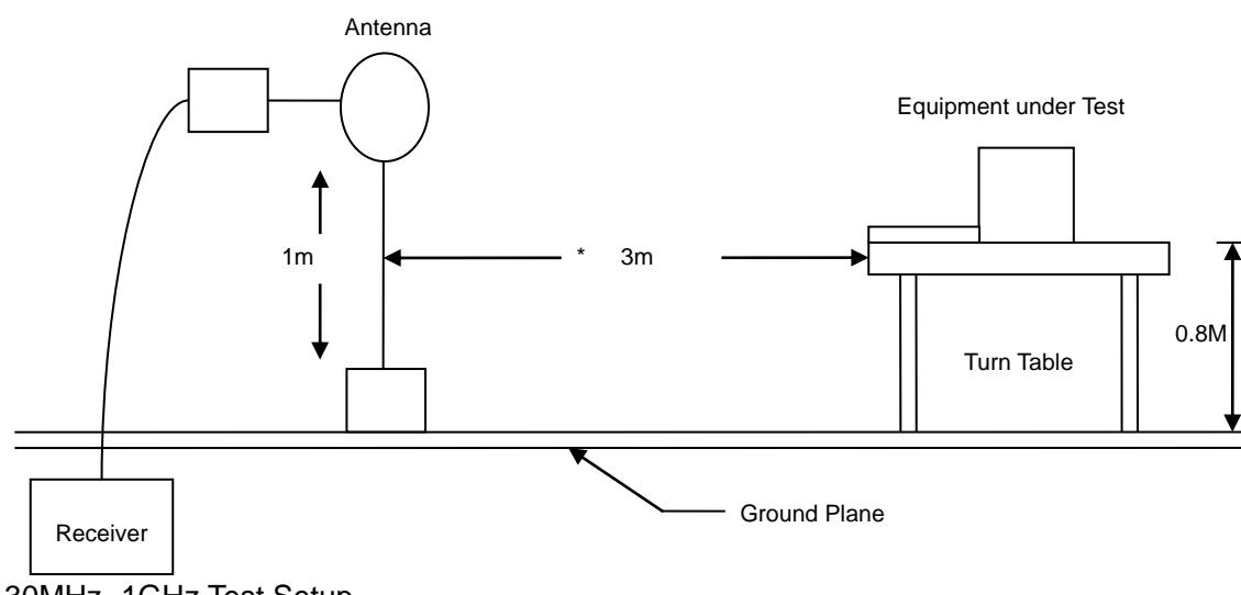
30MHz- 1GHz Test Setup
