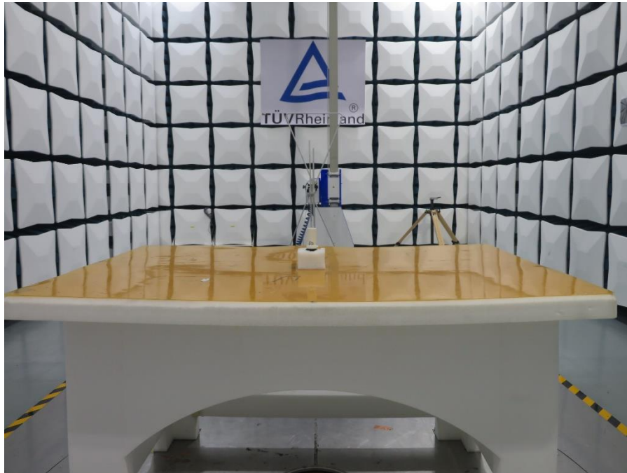
Photograph 1: Set-up for Radiated Spurious Emission, Below 1GHz
