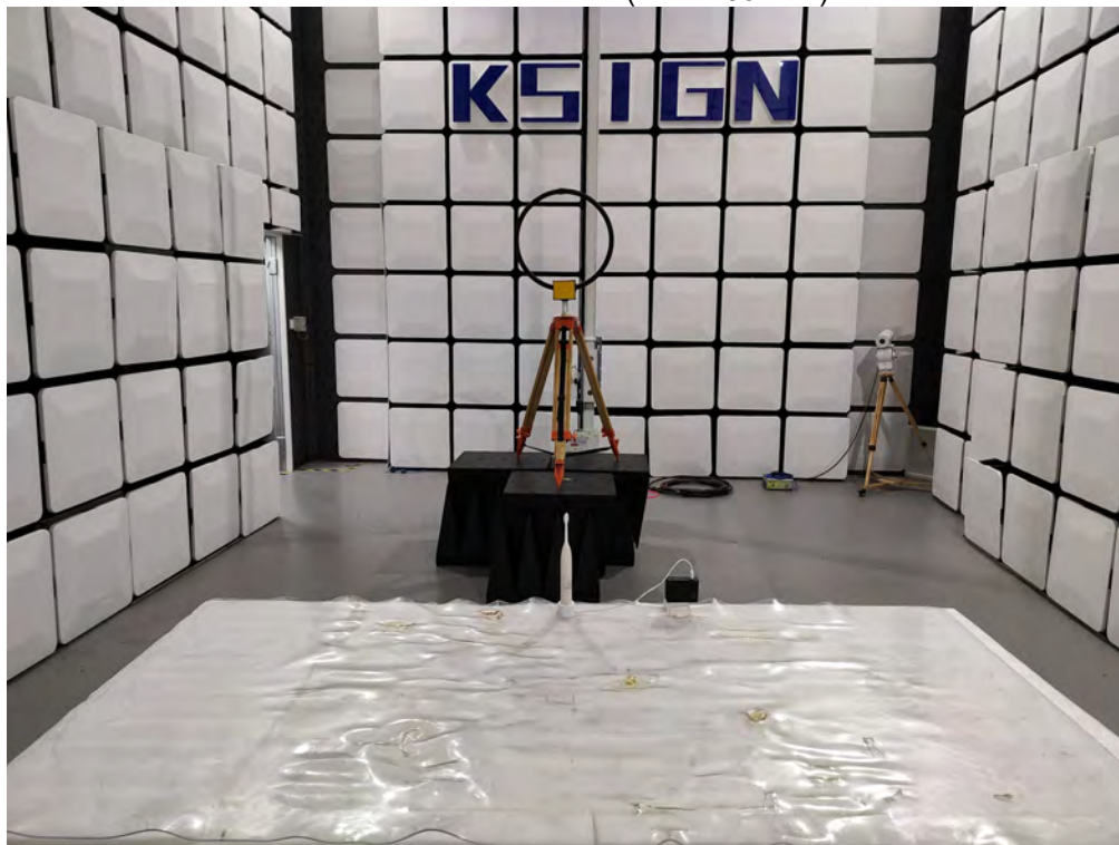
Radiated Measurement (Below 30MHz)
