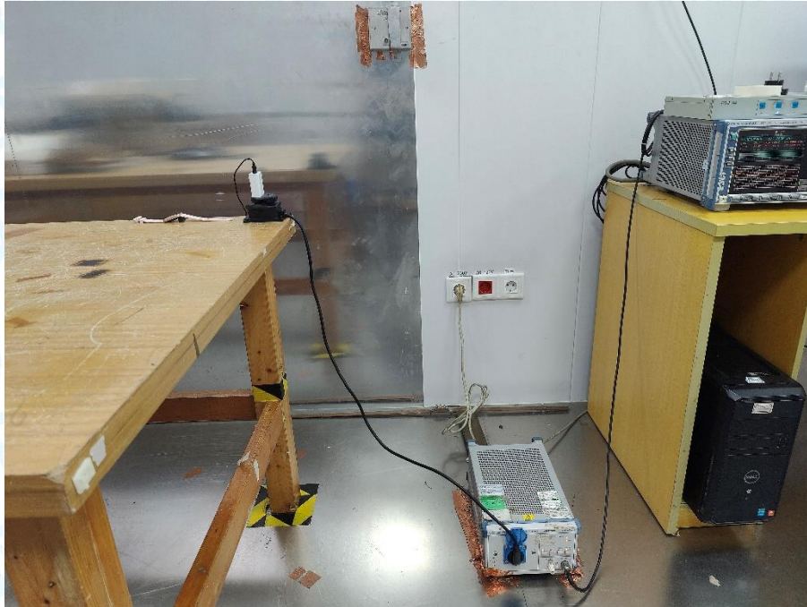
Photo of Setup for Radiated Emission (30MHz~1GHz)
