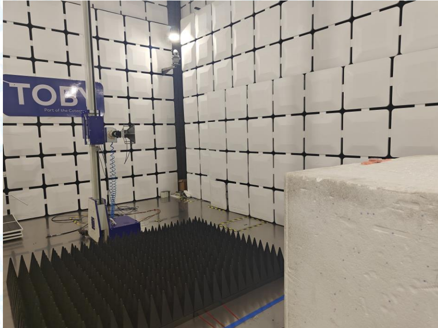
Photo of Setup for Conducted Emission
