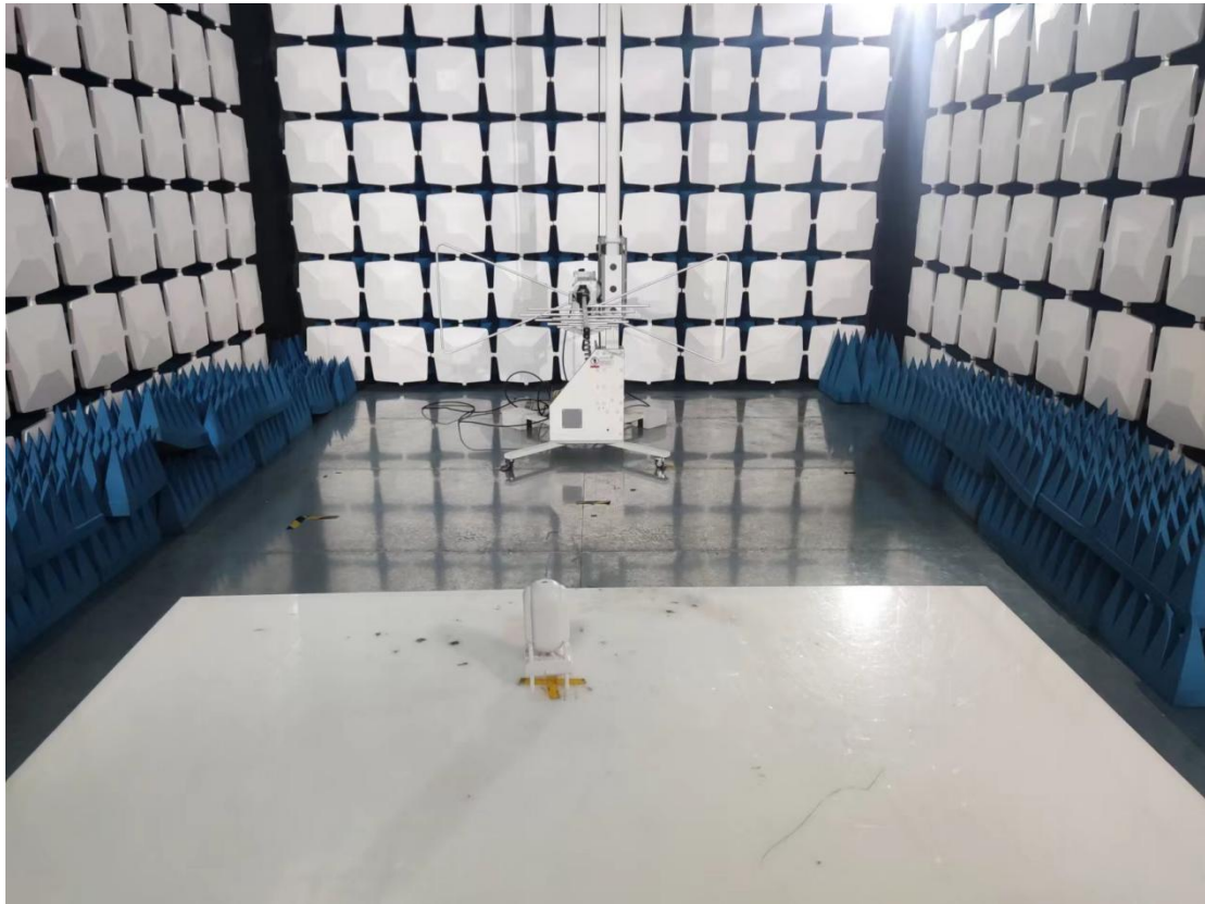
Below 1GHz for radiated emission test setup
