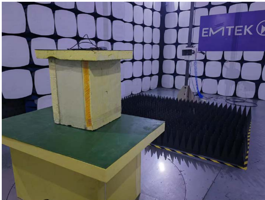
Spurious Emission Test Setup (Above 1GHz)
