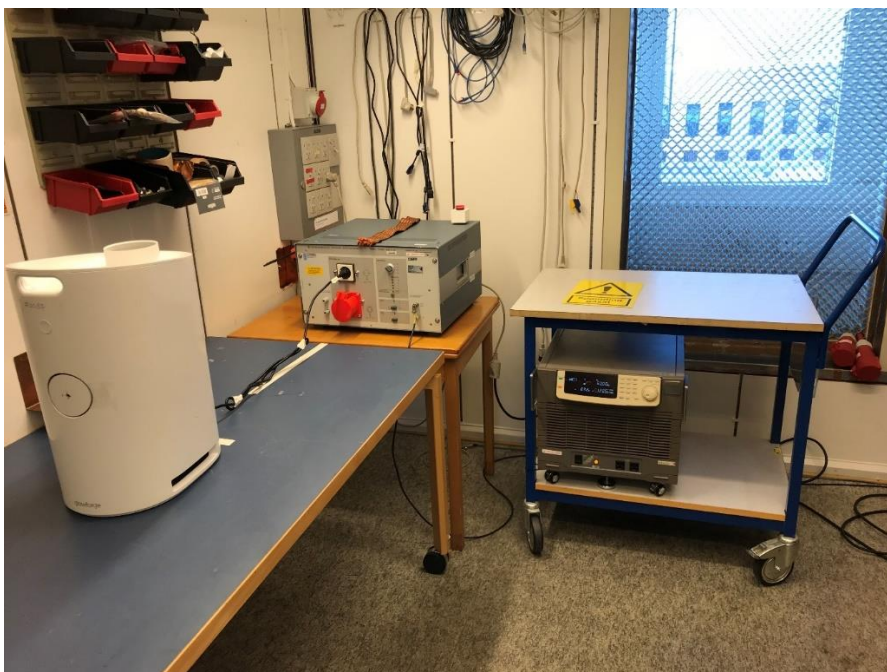
Photo 4.1.1 Measurement of AC power-line conducted emission
