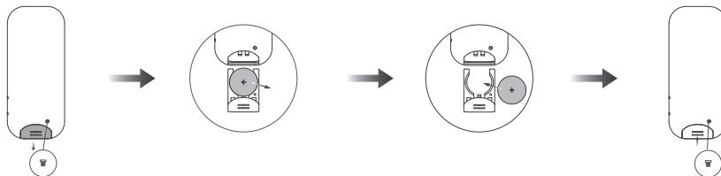
①Loosen the rear cover screws, and slide down to open the battery compartment.
