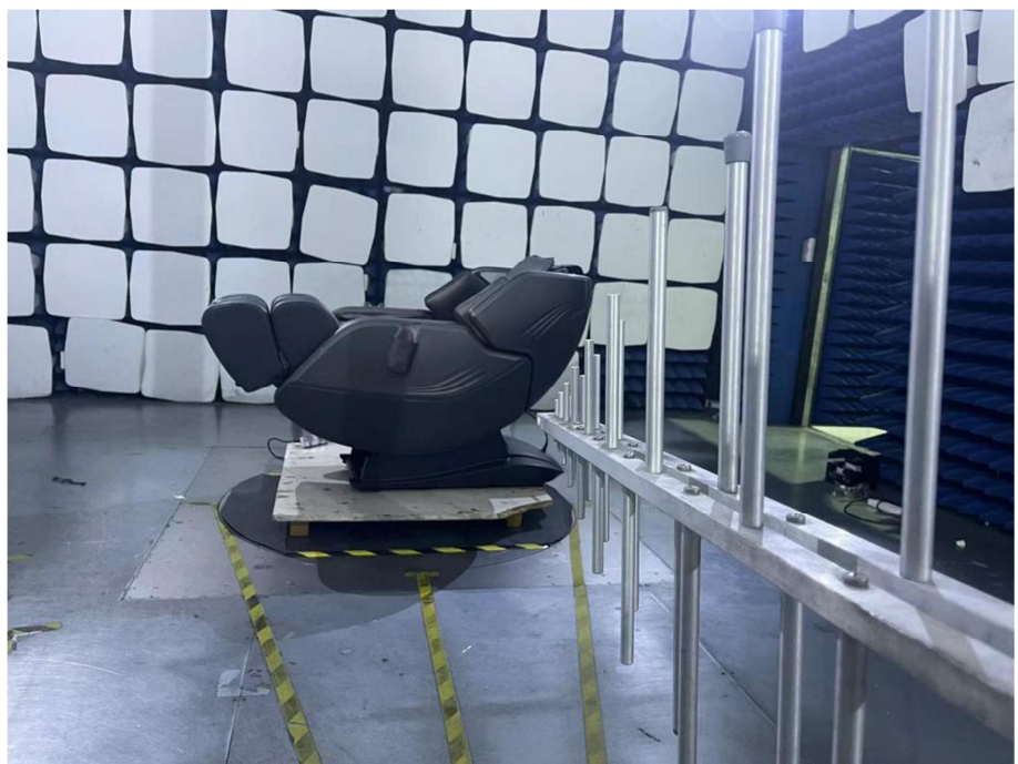
Radiation Emission Test Setup (30MHz to 1GHz)
