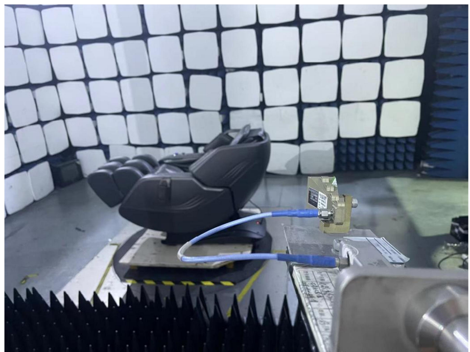
Radiation Emission Test Setup (Above 18GHz)
