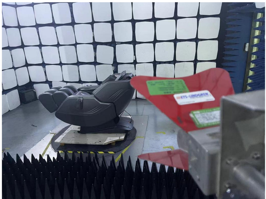
Radiation Emission Test Setup (1GHz to 18GHz)
