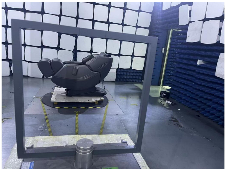
Radiation Emission Test Setup (Below 30MHz)
