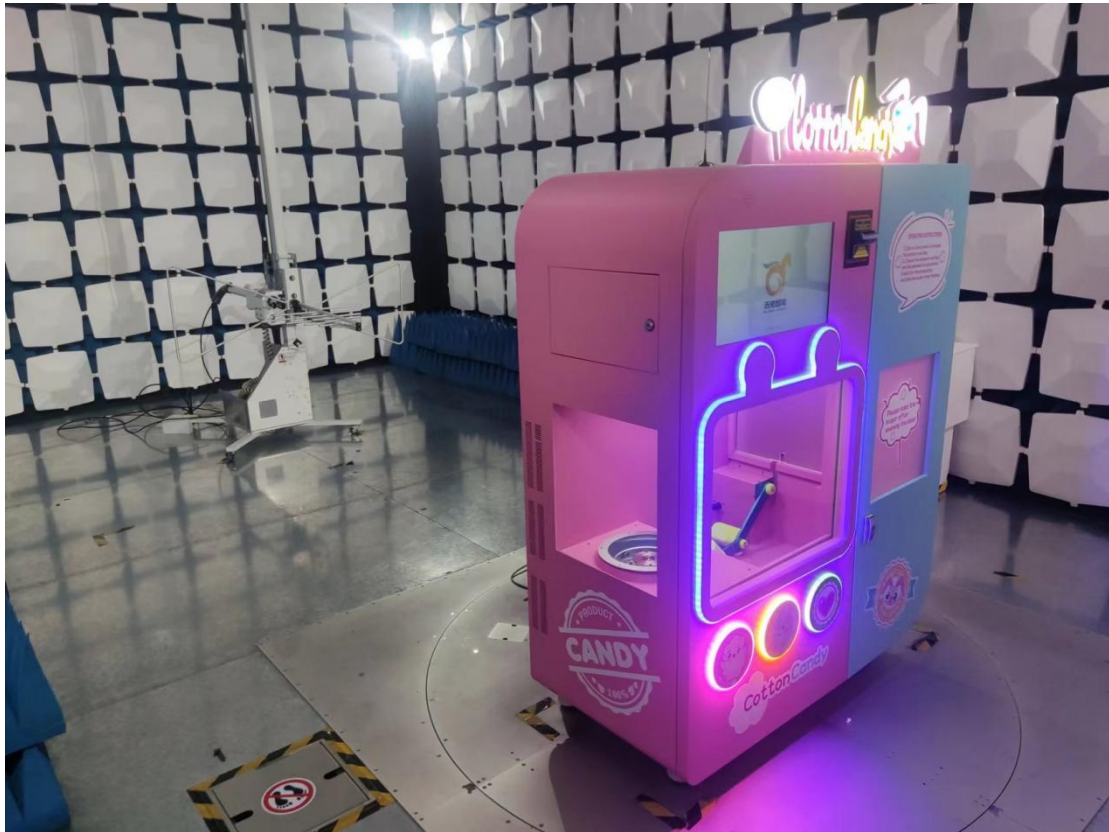
Blow 1GHz for radiated emission test setup
