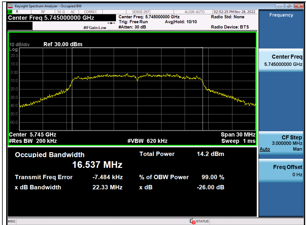
Test_Graph_802.11a_ANT1_5745_6Mbps_OBW
