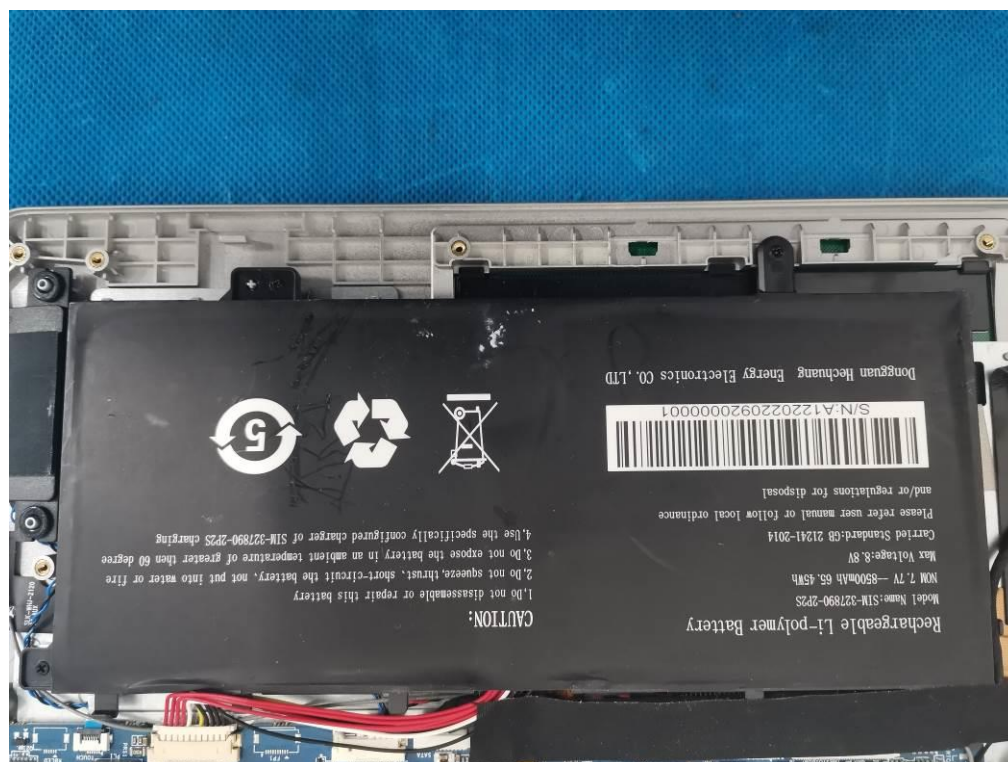
OPEN VIEW OF EUT (FIGURE 6)
