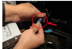
8. Connect original car LVDS cable with carplay box LVDS cable
