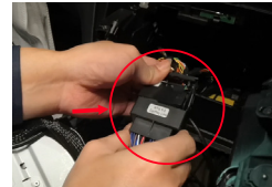
10. Take out the CarPlay 48PIN cable, plug its female side to the original car 48PIN connector.
