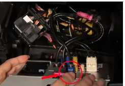
7. Unplug the LVDS cable from multimedia box (most time is a blue head)
