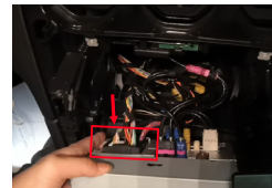
5. Take out the head unit and unplug the original 48PIN main cable
