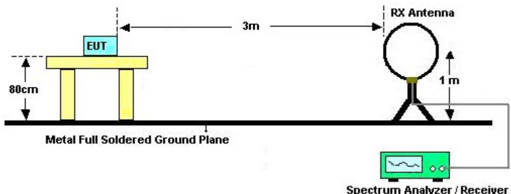
For radiated test from 30MHz to 1GHz
