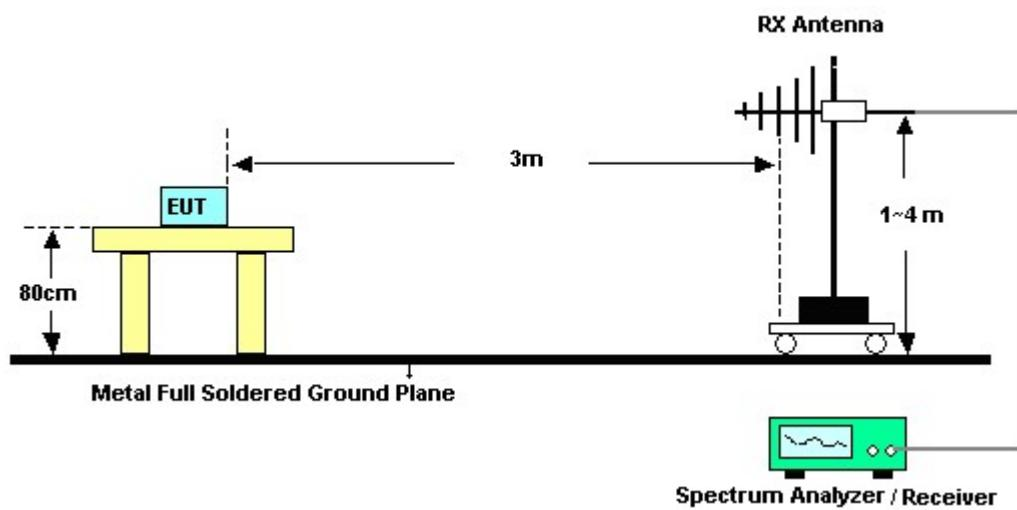
For radiated test from 1GHz to 18GHz
