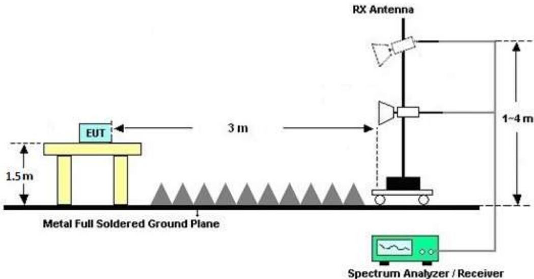
For radiated test above 18GHz
