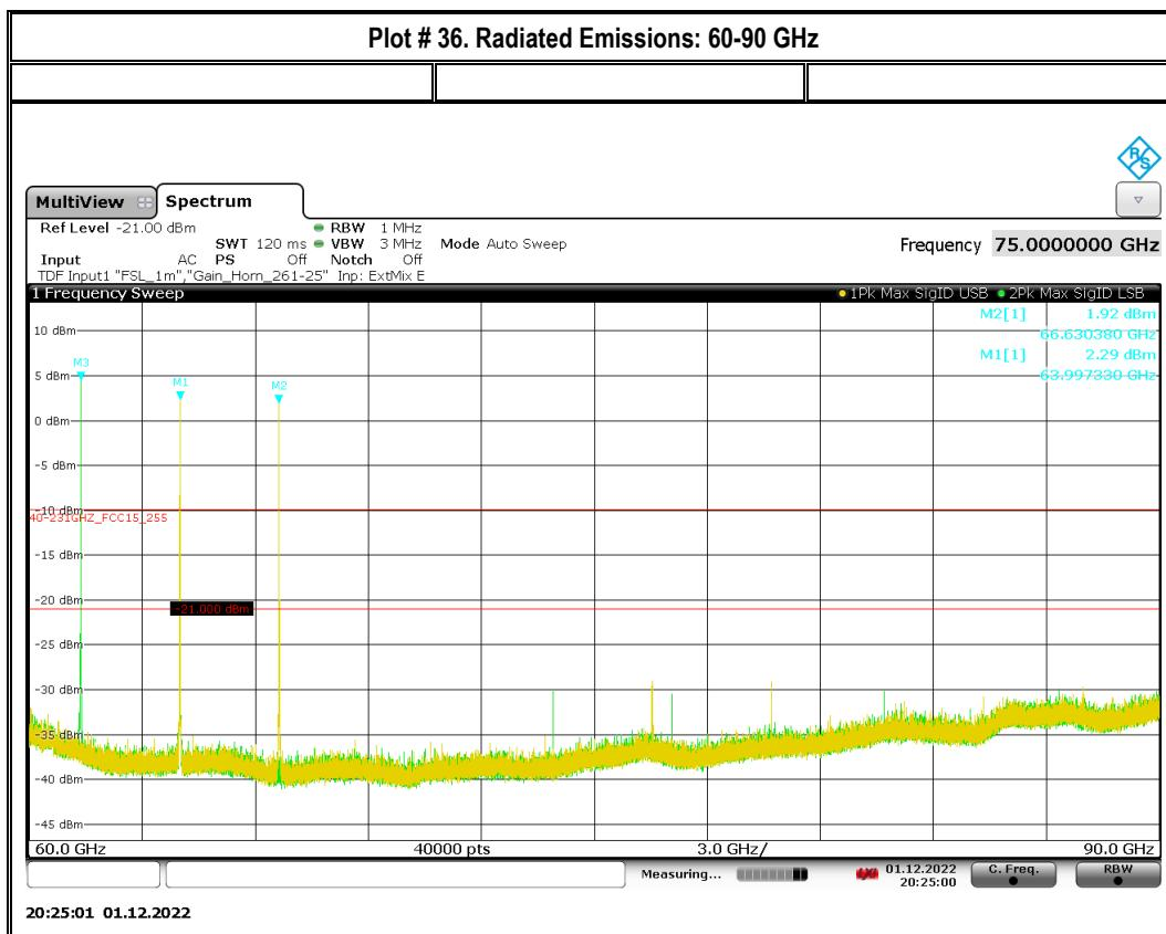
Note: The emission marked by marker 1 is the wanted emission. The one at marker 2 is investigated in the following diagram. The emission at marker 3 shows no trace-overlapping, thus image signal.
