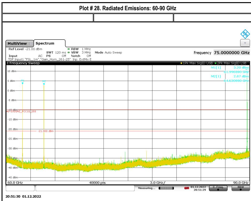
Note: The emission marked by marker 1 is the wanted emission. The emissions at marker 2 and 3 shows no trace-overlapping, thus image signal.
