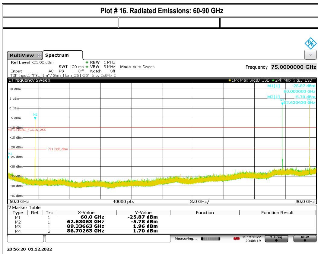
Note: The emission marked by marker 1 is the wanted emission. The ones at marker 2 and 3 are investigated in the following diagrams. The emission at marker 4 shows no trace-overlapping, thus image signal.
