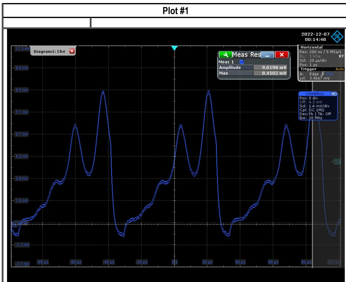
Note: measured with the DSO, shows max. voltage = 8.45 mV at a distance of 7 cm to EUT.
