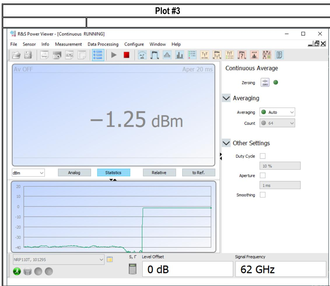
Note: measured the conducted power from the signal generator of -1.25 dBm.
