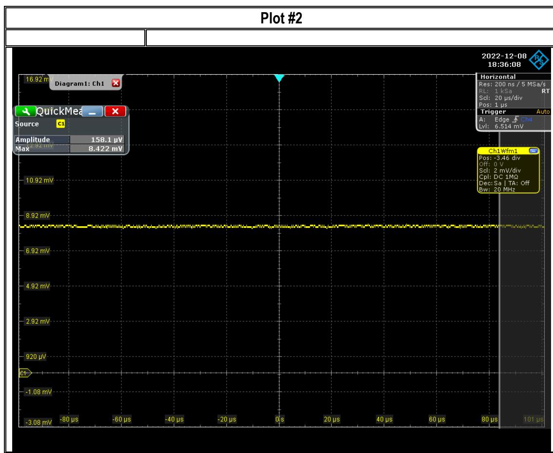
Note: reproduce the max. voltage level of 8.42 mV with a signal generator and transmitting antenna at a distance of 62 cm.
