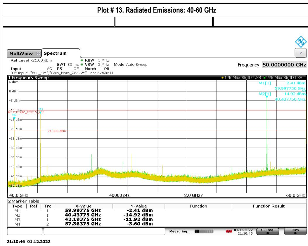
Note: The emission marked by marker 1 is the wanted emission. The ones at marker 2 and 3 are investigated in the following diagrams. The emission at marker 4 shows no trace-overlapping, thus image signal.
