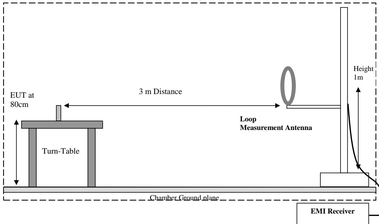
Radiated Emissions Test Setup 30MHz-1GHz Measurements
