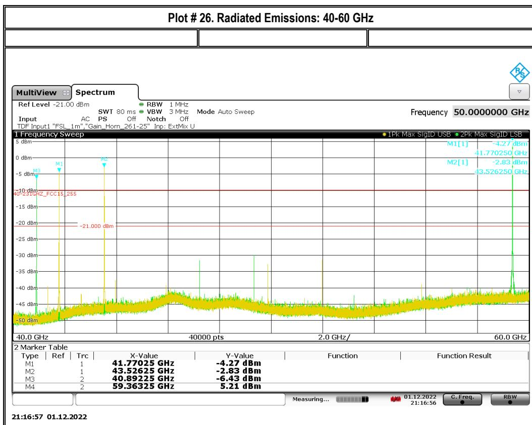
Note: The ones at marker 1 and 2 are investigated in the following diagrams. The emissions at marker 3 and 4 show no trace-overlapping, thus image signal.
