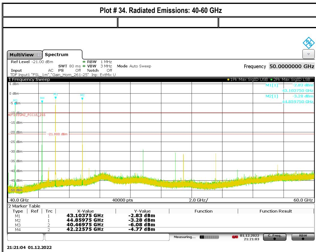
Note: The ones at marker 1 and 2 are investigated in the following diagrams. The emissions at marker 3 and 4 show no trace-overlapping, thus image signal.
