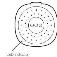
The Lumos Firefly has a small LED indicator to convey different information. Please note the colours below and the corresponding message.
