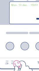
Refer to the "**Use**" section on page 6 for badging. Badge the terminal, the screen displays **the current date and time**, the test is successful, proceed to step 3.
