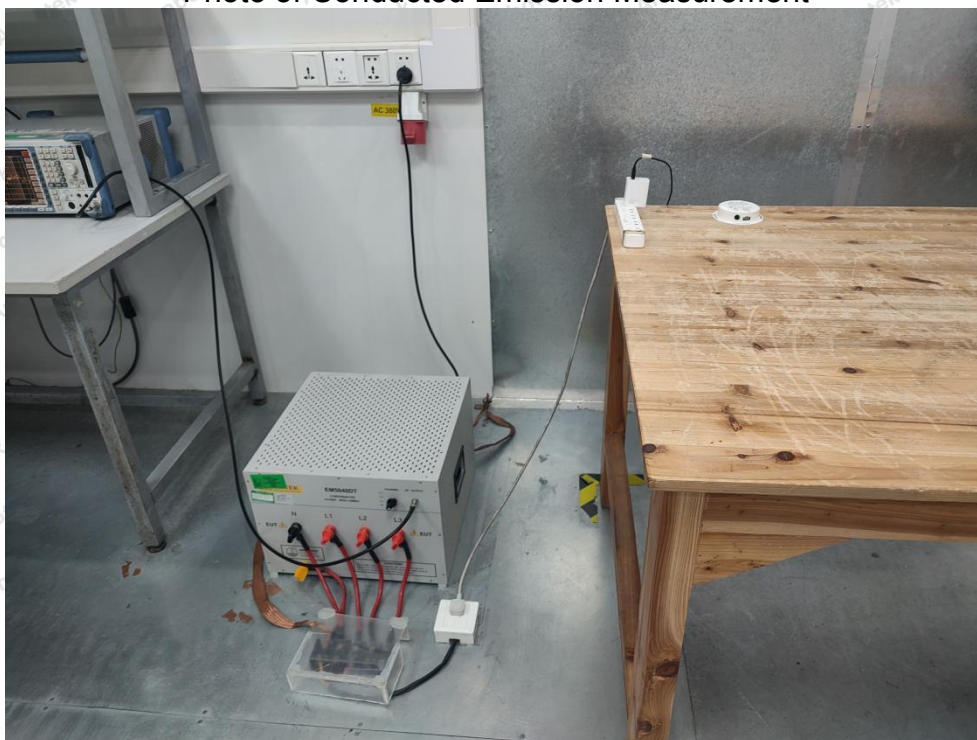
Photo of Conducted Emission Measurement
