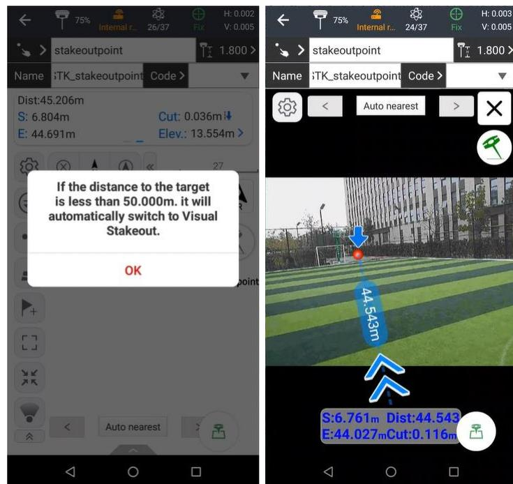
(7) If the distance to the target is less than 3.0m meters, it will automatically switch to Vision Stakeout. (with Bottom Camera)
