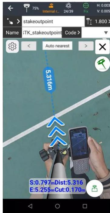
(8) After we are within 1cm from the target point, we can click the measurement icon to collect
