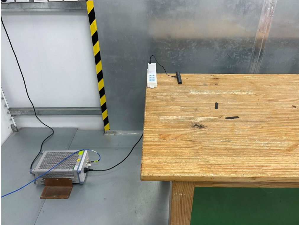
AC Power Line Conducted Emission
