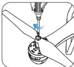
**Installation:** The drone will not fly unless the correct propeller is installed on the correct motor shaft. Each propeller is labeled with either an "A" or "B" on it. Secure the propeller onto the motor shaft using screws, turning each screw clockwise.
