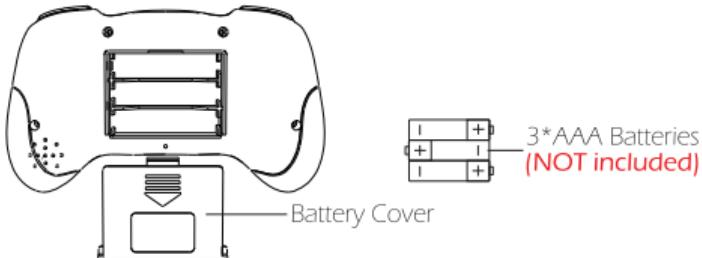
Open the battery cover on the back of the transmitter, insert the three AAA batteries **(Not included)** into the battery compartment, and close the battery cover to complete the installation.
