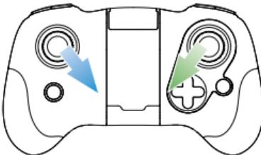
Simultaneously push the left joystick to the bottom right corner and the right joystick to the bottom left corner. The motors will rotate, and the drone is unlocked.
