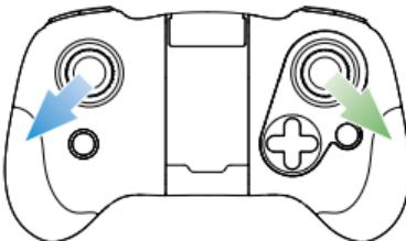
Push the left and right joysticks simultaneously to the outer, lower corners to calibrate the gyro. The drone indicator will blink and turn solid, the transmitter beeps one time, indicating that the calibration is completed.
