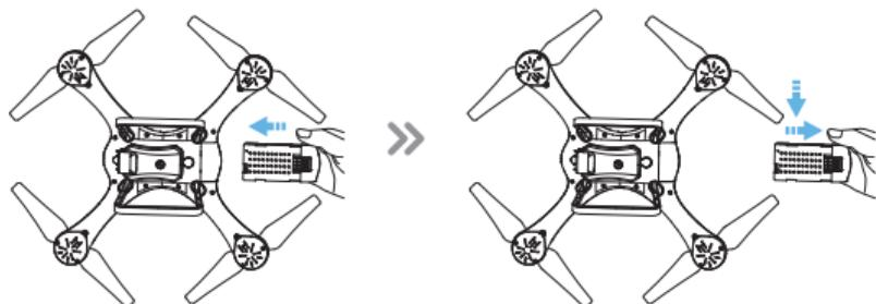
**Installation:** As shown in the figure above, align the battery and insert it into the bottom of the drone. Make sure the battery buckle is secure.
