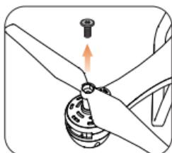
**Removal:** For propeller removal, use a screwdriver(provided) to rotate the screws counter-clockwise and remove the propellers
