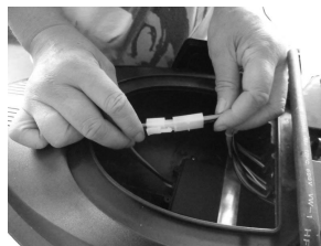
2 Connect the battery plug with the socket in the boat
