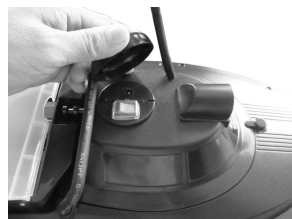
5 Turn on the power switch and both tail lights start to flash.
