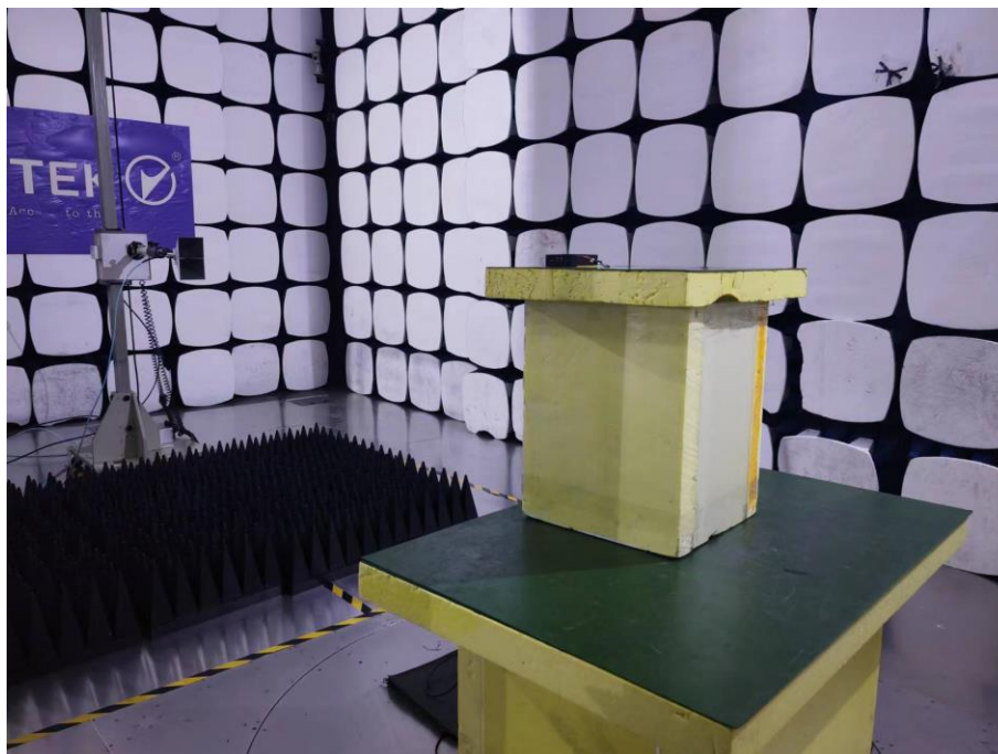
Spurious Emission Test Setup (Above 1GHz)
