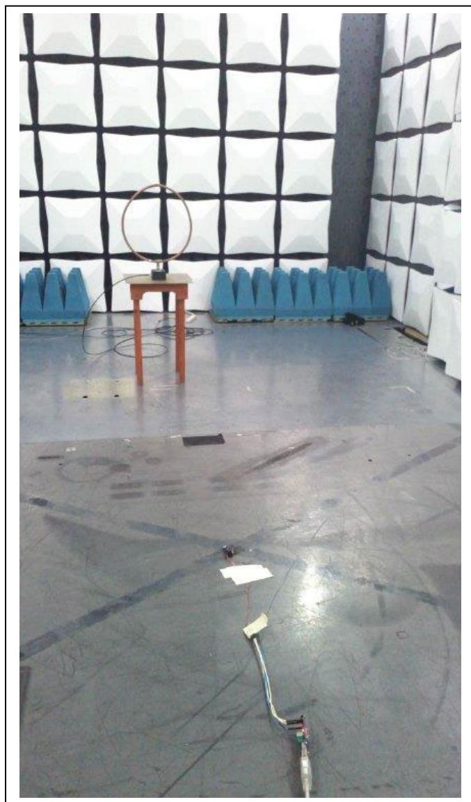
**Radiated Spurious Emissions 30 MHz to 1000 MHz**
