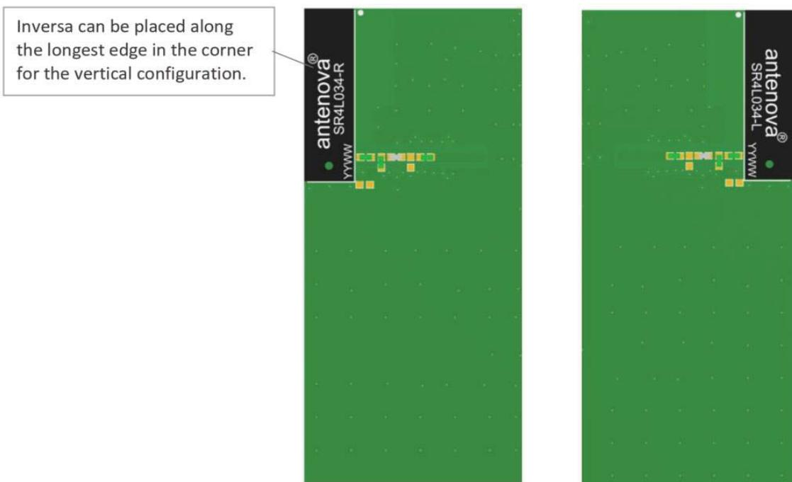
Note: Vertical placement optimal minimum GND length required is  $\geq 100\text{mm}$
