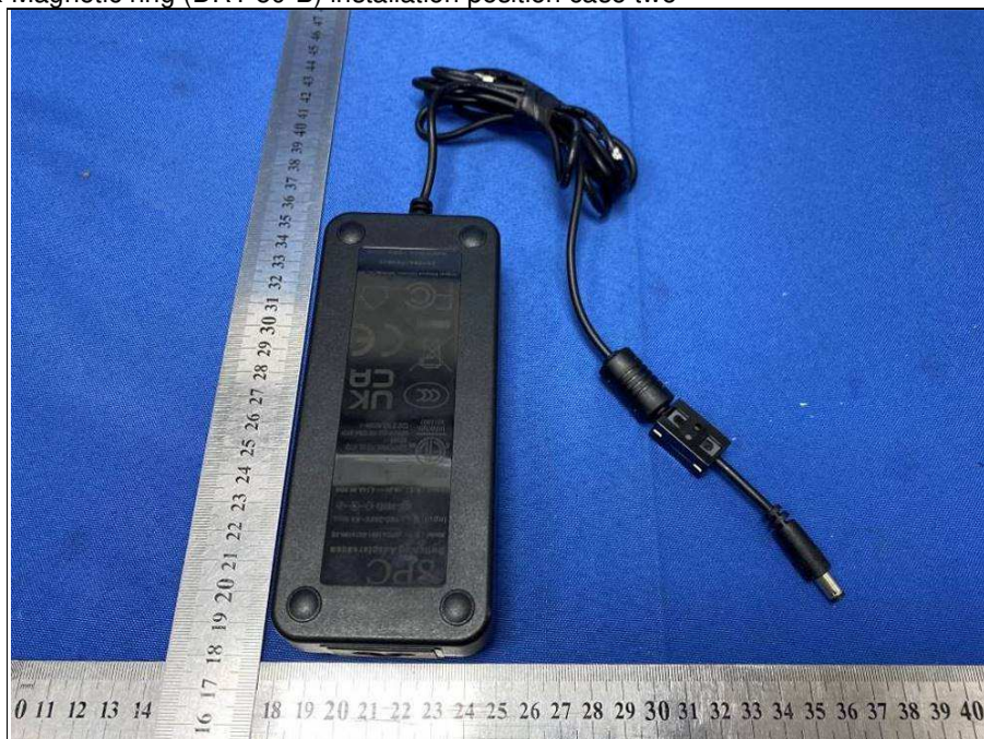
Adapter 2 & Magnetic ring (DRY-50-B) installation position case two
