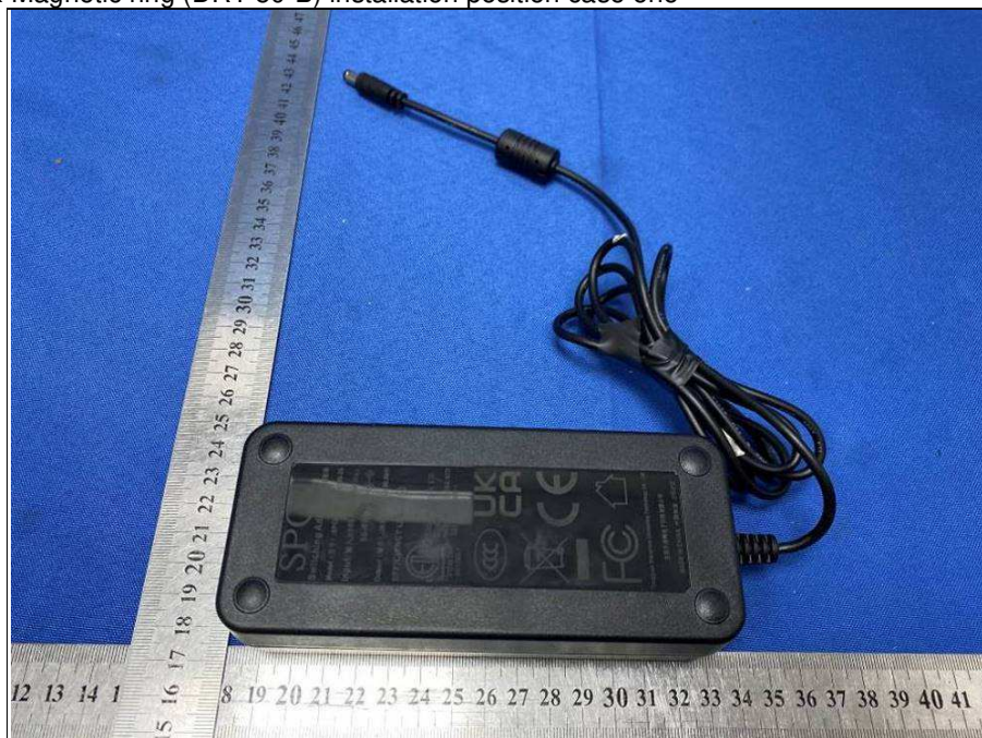
Adapter 2 & Magnetic ring (DRY-50-B) installation position case one
