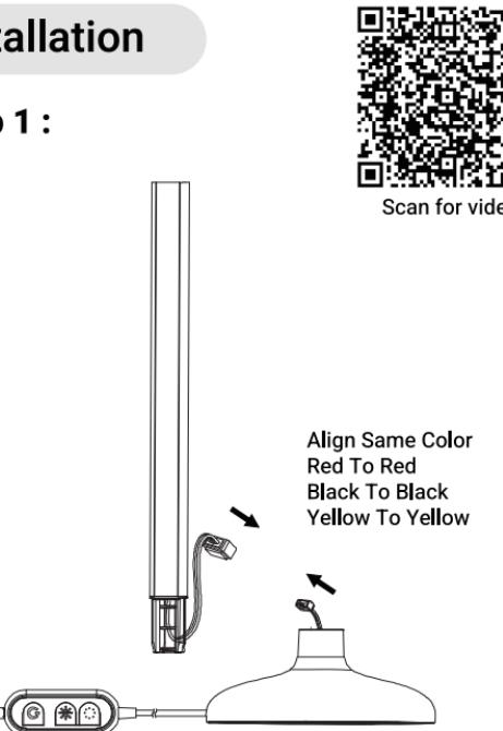
Connect the wire interface between the lamp base and led tube 4
