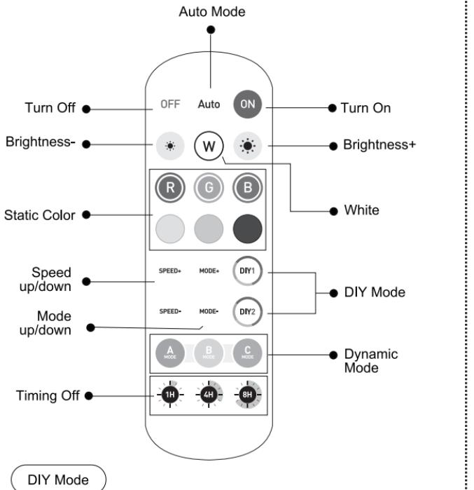
Long press DIY key to save light state(color/mode) to the DIY key. After that, short press the DIY key to call it.
