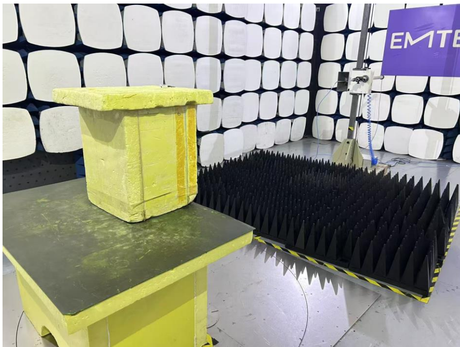
Spurious Emission Test Setup (Above 1GHz)
