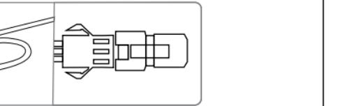
Step2: Connect the LED Controller with power supply.
