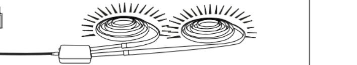
One or two LED strips use a universal controller, and both ports have the same functionality; either port can be used for insertion.
