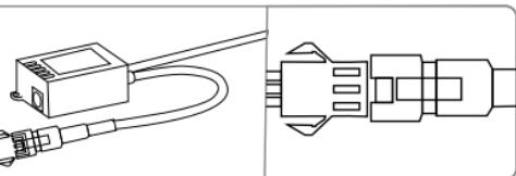
Step2: Connect the LED Controller with power supply.
