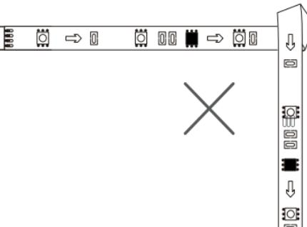
Recommended Tip: Try not to bend at electronic components like light beads, bonding pad to avoid short circuit.
