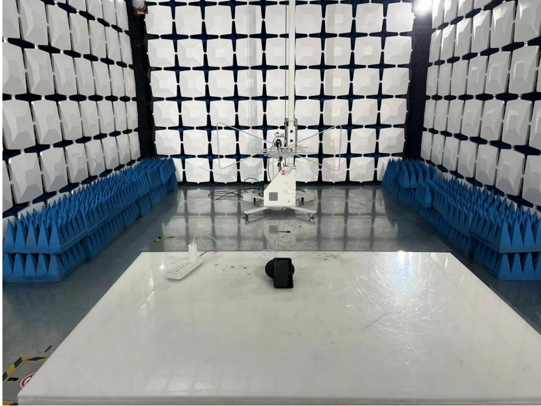
Blow 1GHz for radiated emission test setup
