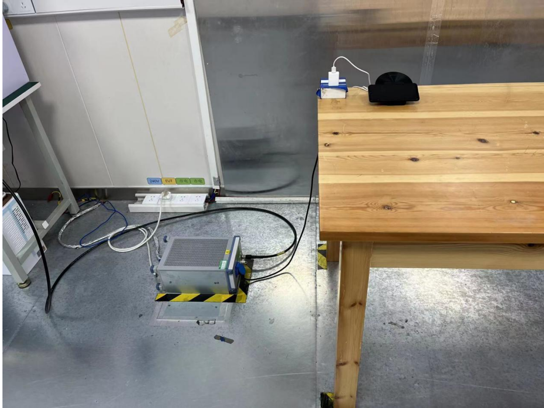
Conducted emission test setup
