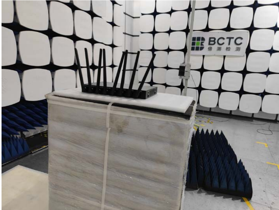
Spurious Emission Test Setup (Above 1GHz)
