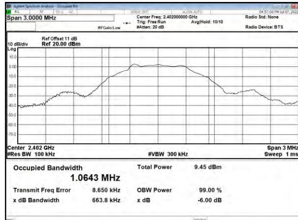
Modulation Type: GFSK(125kbps)
