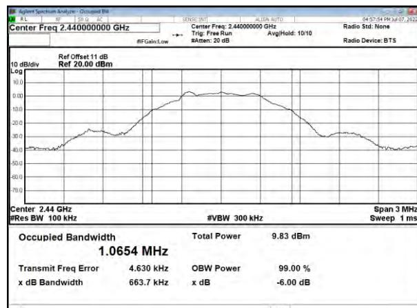
Modulation Type: GFSK(125kbps)
