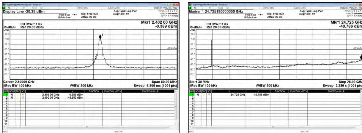
Modulation Type: GFSK(125kbps)
