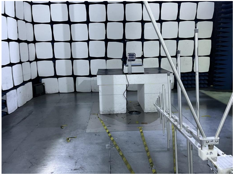
Radiation Emission Test Setup (30MHz to 1GHz)
