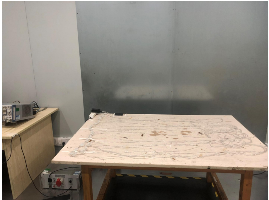
Conducted Emission Test Setup
