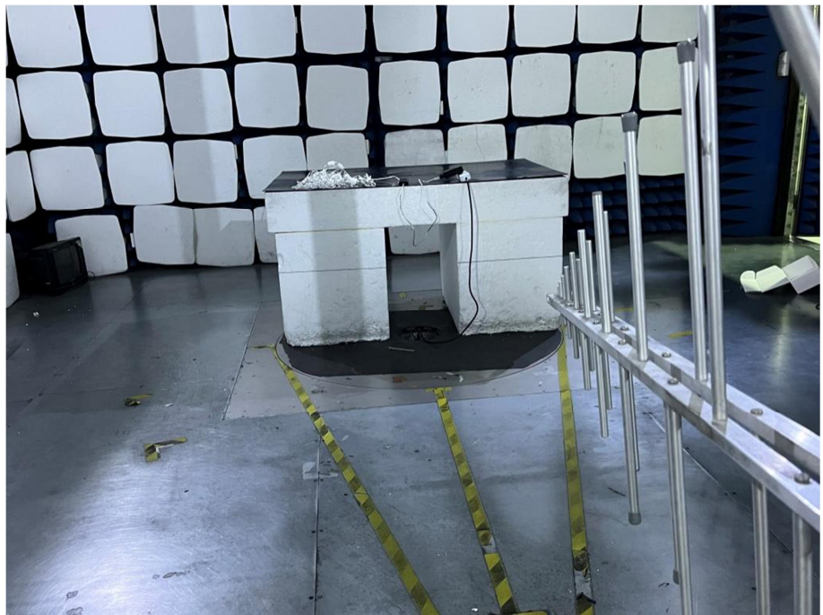
Radiation Emission Test Setup (30MHz to 1GHz)
