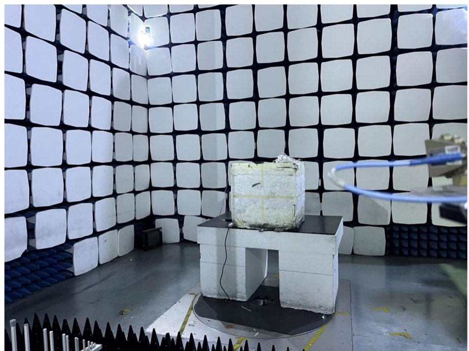
Radiation Emission Test Setup (Above 18GHz)
