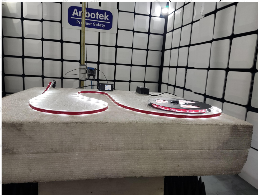
Photo of Radiation Emission Test (Above 1GHz)
