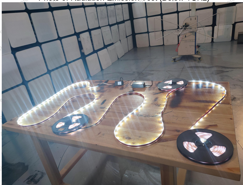
Photo of Radiation Emission Test (Below 1GHz)
