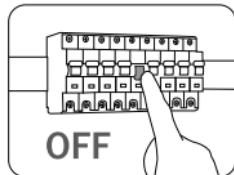
② Use an electric tester pen or voltmeter to test the circuit. Make sure there is no power before operating.
