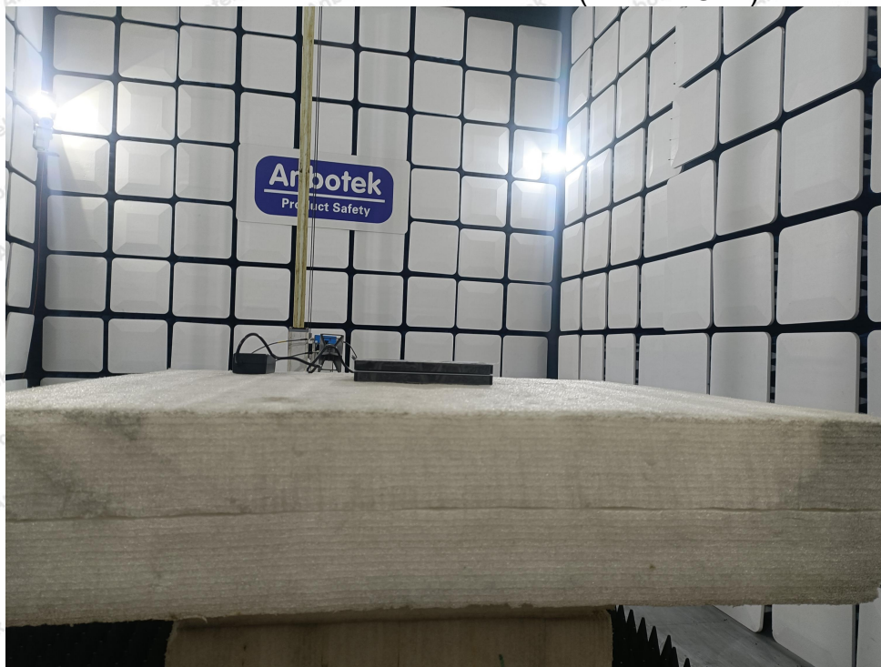
Photo of Radiation Emission Test (above 1GHz)
