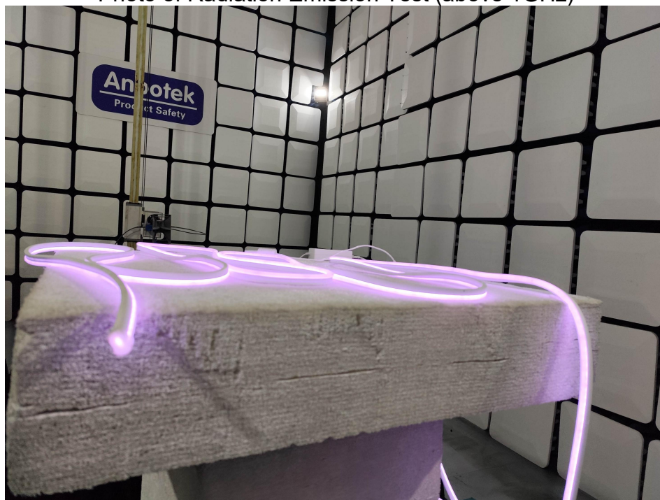
Photo of Radiation Emission Test (above 1GHz)
