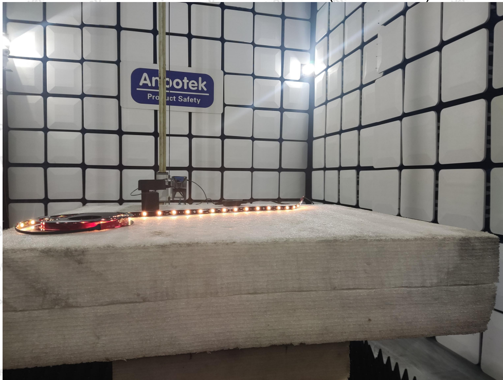
Photo of Radiation Emission Test (above 1GHz)
