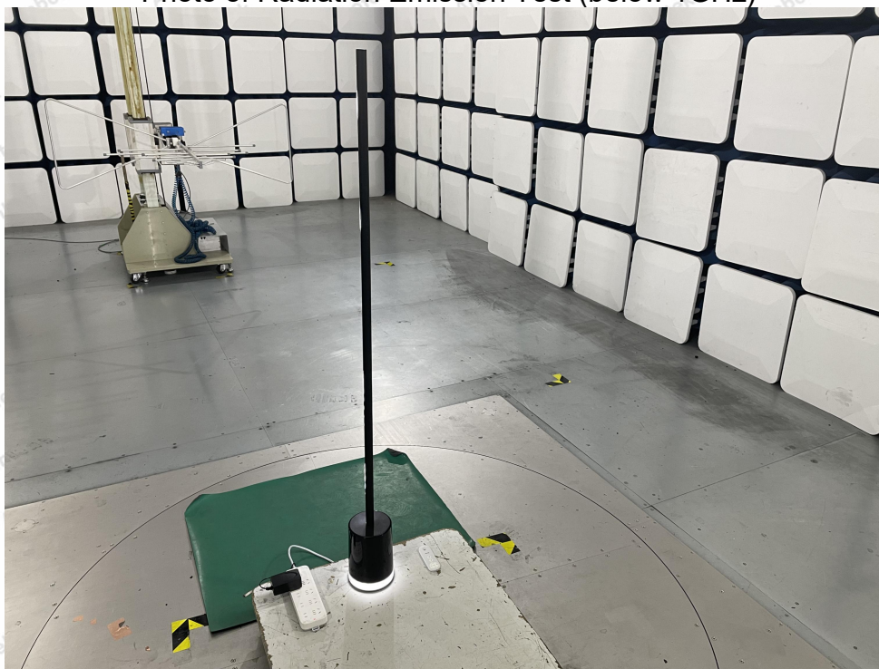
Photo of Radiation Emission Test (below 1GHz)
