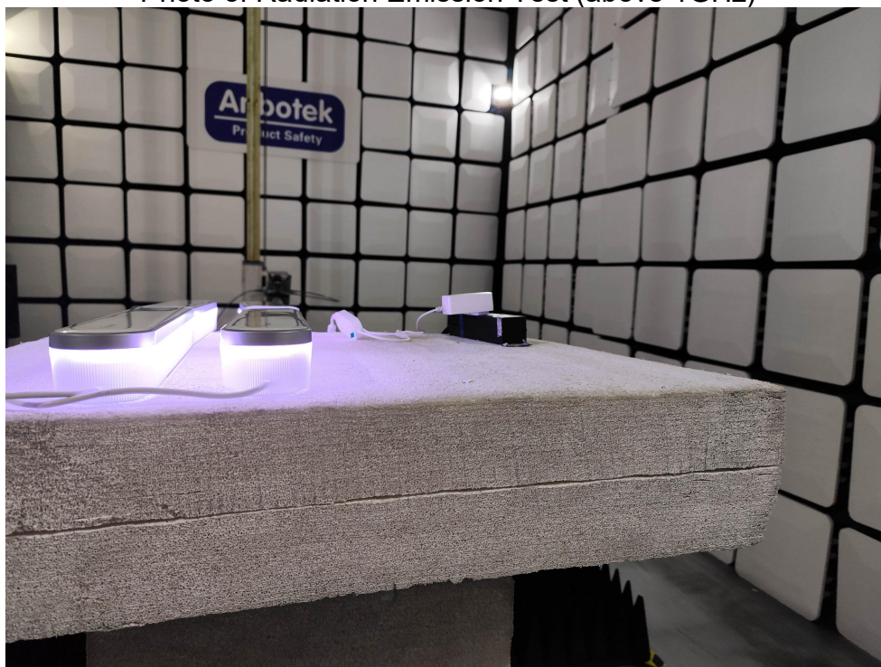
Photo of Radiation Emission Test (above 1GHz)
