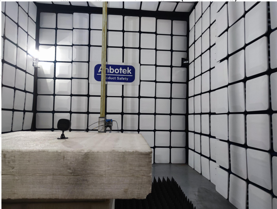
Photo of Radiation Emission Test (above 1GHz)
