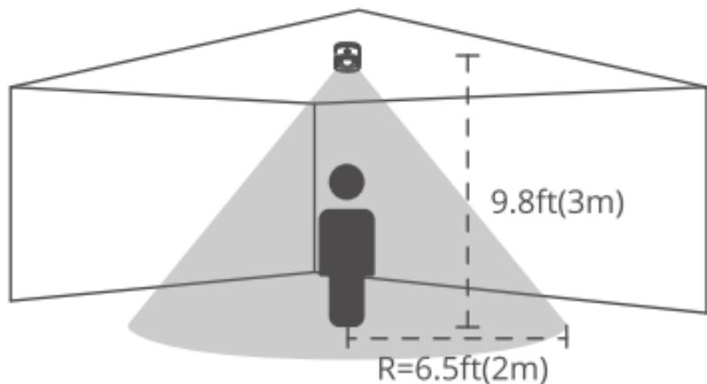
b. **Installing on the Ceiling:** If the ceiling is 9.8ft (3m) high, the detection range will be a circle with a radius of 6.5ft (2m) on the ground. Advantages: It is good for detecting static targets that are sleeping. Disadvantages: The detection range is small.
