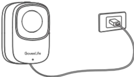
2. When the device is powered on, the indicator will become solid, which means the device has entered the Bluetooth Broadcast Mode. Search H5127 in the app. Follow the in-app instructions to press the function button when the indicator is flashing to complete pairing.
