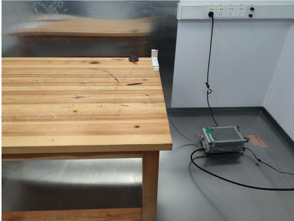
Photo of Conducted Emission Measurement
